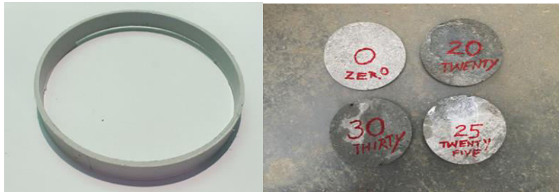
Fig. 1: Mould used for specimen preparation Fig. 2: Specimens used to find the thermal conductivity
