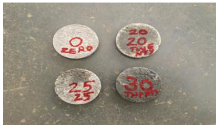
Fig. 3: Specimens used to find the Specific heat Fig. 4: Specimens used to find Thermal expansion
