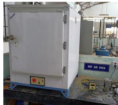
Fig. 6: Test set up for the determination of specific heat
