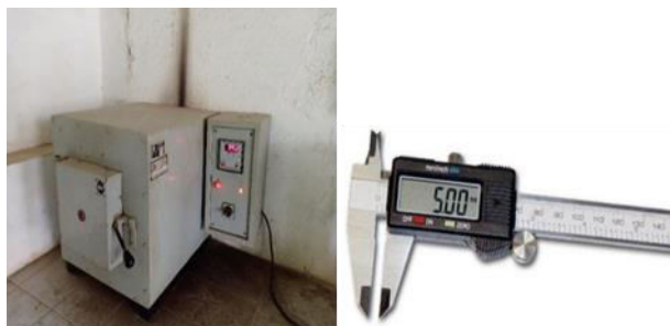
Fig.7: Test setup for the determination of Thermal Expansion
